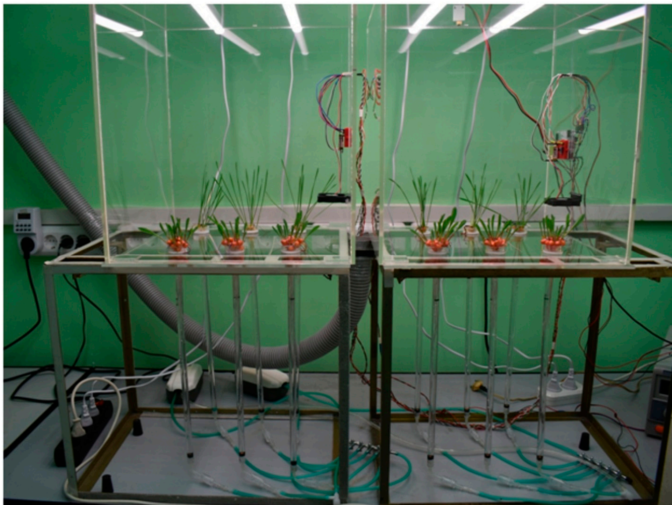
Figure 1. Climatic plant growth chambers with control of temperature, humidity, and carbon dioxide concentration with the possibility of interfacing with NMR equipment to study the state of the plants' hydraulic systems under controlled stress and environmental conditions.
