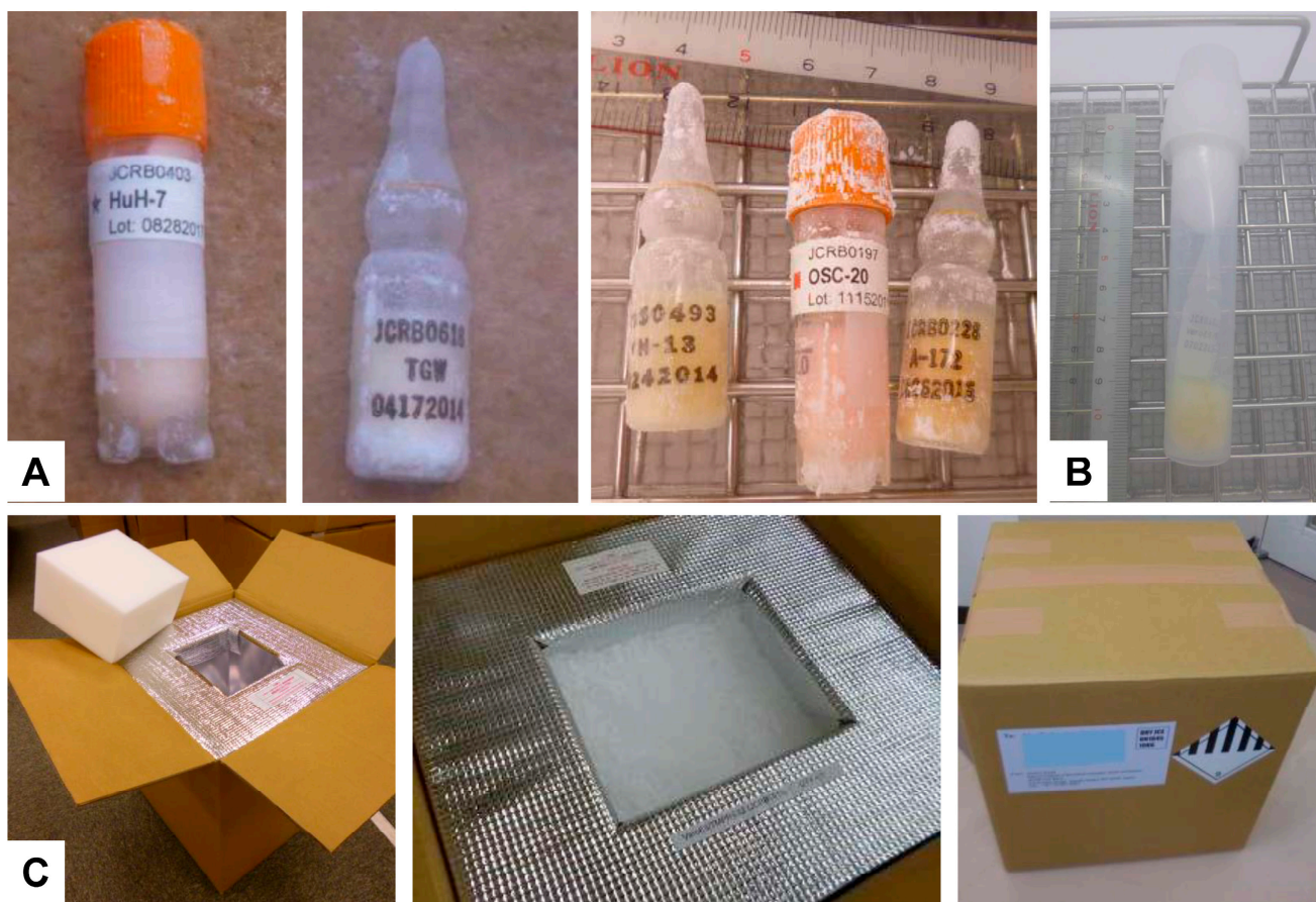
Figure 7. Parceling of frozen cells for transport. (A) Various glass or plastic storage vials containing frozen cells prepared for dispatch are depicted. (B) A secure container designed to hold the vials during transit is shown. (C) The packaging process is highlighted, emphasizing the use of dry ice to maintain the low temperatures essential for preserving cell viability.
