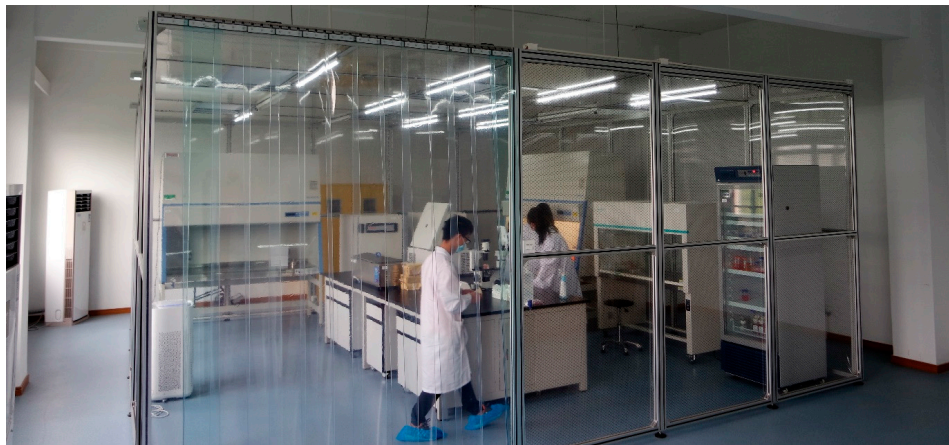
Figure 4. The Shanghai University (SHU) iSmart Institute cell culture room for the organ-on-chip (OoC) experiments. The area is isolated, with the high efficiency particulate air (HEPA) filtration, temperature and humidity control. The air pressure inside is kept positive to keep away the outside air. The cell culture room has an area of 30 m 2 (5 × 6 m) and accommodates the instruments necessary for work: refrigerators, freezers, cell culture incubators, biological safety cabinet, microscope, and chip setup with fluid control.
