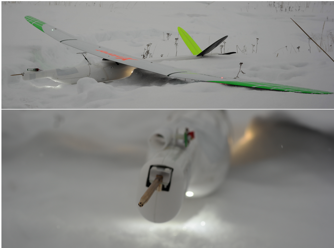
Figure 3. MASC with enlightening (top). Picture of the probe tip (bottom).
