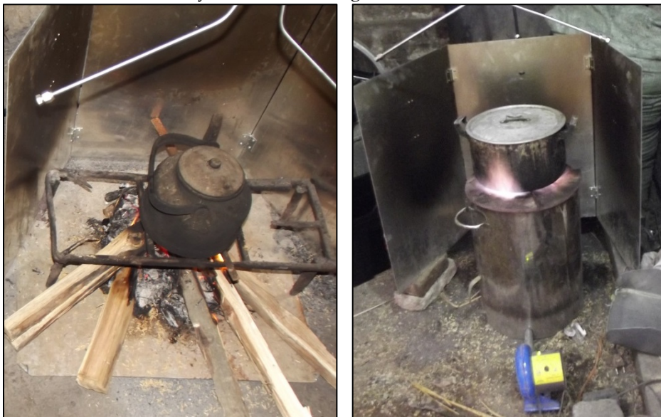
Figure SM16. North Vietnam: Traditional North Stove (left), and Rice Husk Gasifier (right) with the blower fan housed in the blue and yellow casing.
