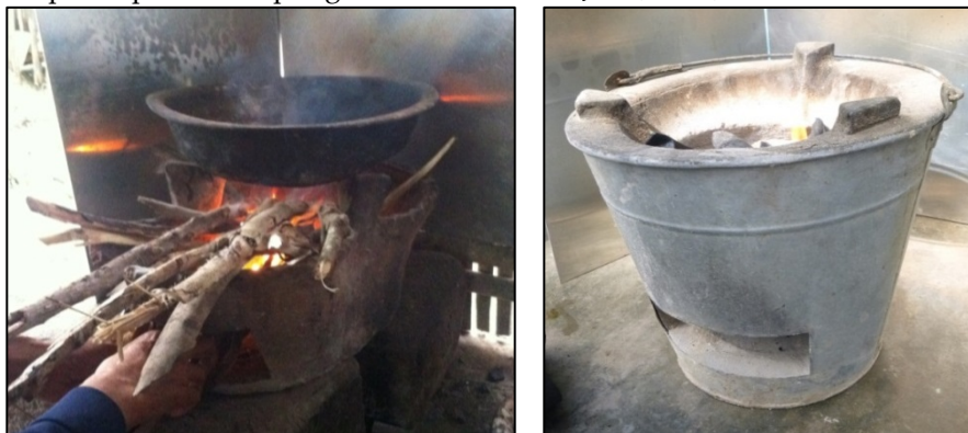
Figure SM15. South Vietnam Stoves: Traditional Mekong Delta Wood Stove (left) and the “High Efficiency Stove” or HES (right).
