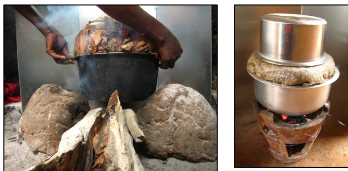
Figure SM12. Three-stone-fire (left) and traditional ceramic charcoal stove (right) in Uganda.
