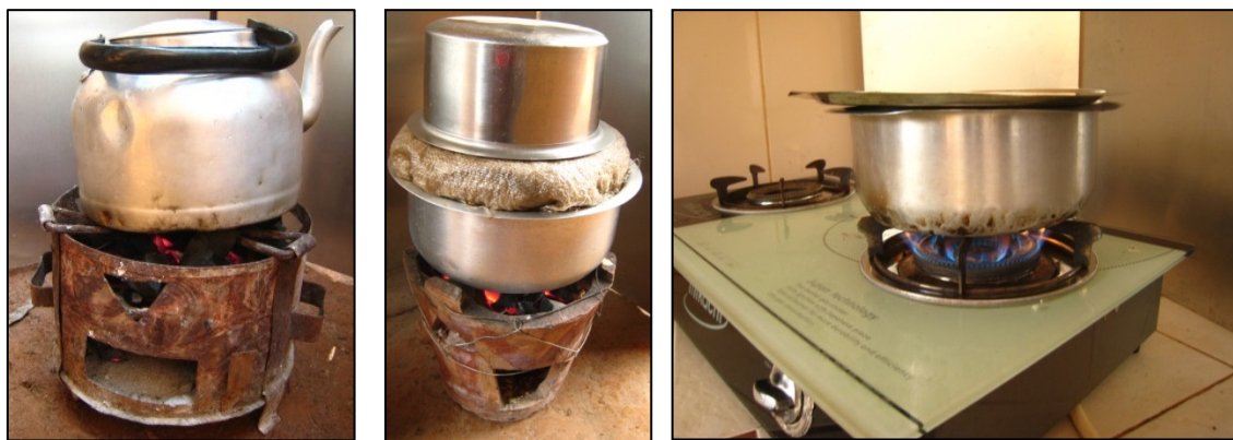
Figure SM8. Ugandan metal charcoal stove (left), traditional ceramic charcoal stove (middle) and an LPG two-burner stove (right).
