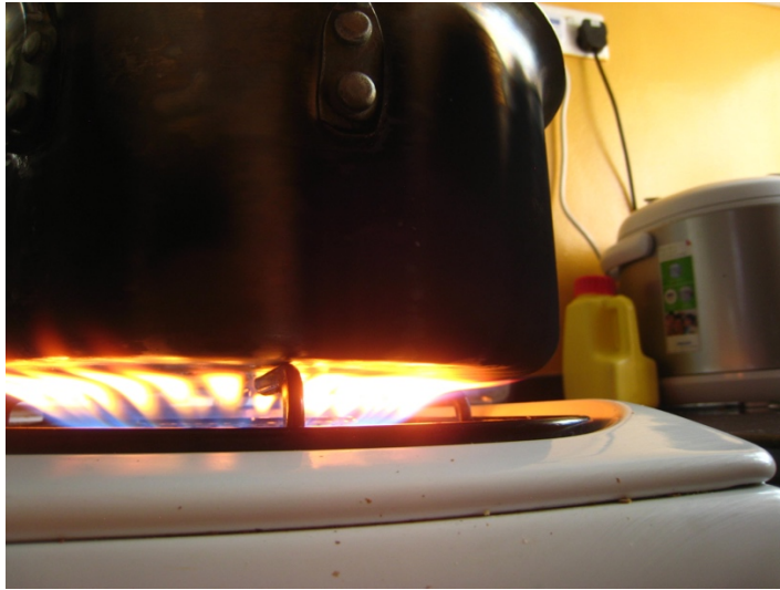
Figure SM21. Example of an LPG stove with a yellow flame, one of three samples which had detectable PM_{2.5} emissions.
