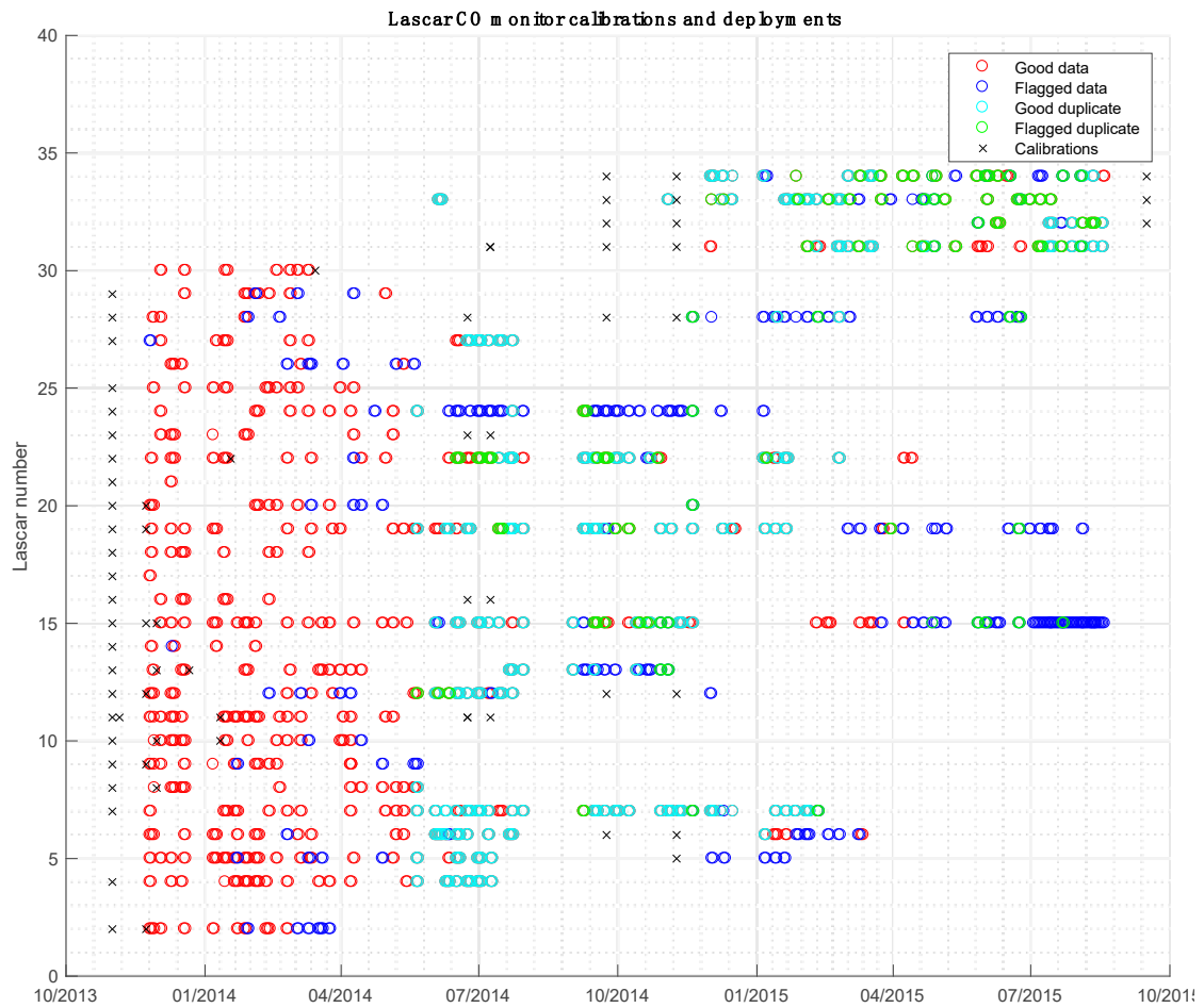
Figure S4. Lascar USB-CO calibration and data quality time line. Some Lascar monitors like #1 and #3 never operated correctly and were returned to the manufacturer. In most cases, the monitors were non-operational upon their return to the CU Boulder Hannigan Lab, so a post-calibration could not be performed.
