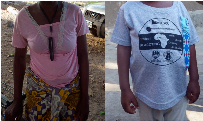
Figure S1. Lascar CO monitors worn on lanyards around the neck or placed inside custom pockets on project t-shirts.
