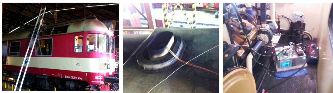
Figure 5. Series 854 diesel-hydraulic railcar tests: installation of the sampling line (left); sampling probe (middle); and portable emissions monitoring system (right).
