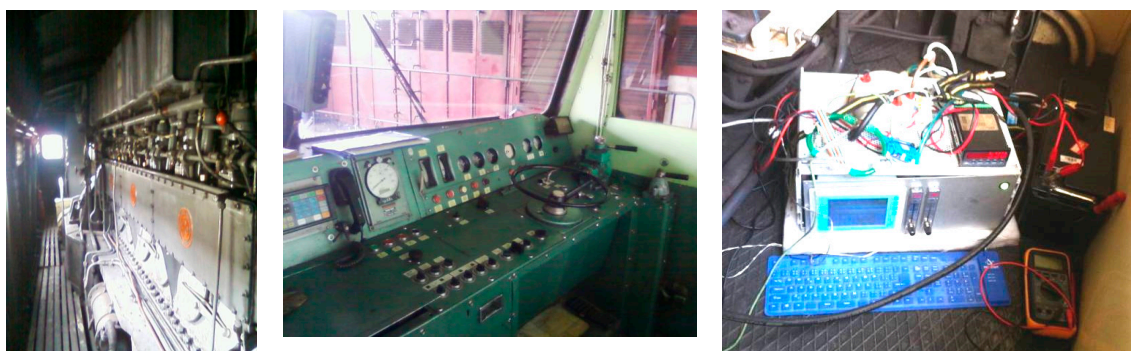
Figure 3. ČKD Series 749 diesel-electric locomotive: ČKD K 6 S 310 DR engine (left); locomotive controls (middle); and portable emissions monitoring system (right).
