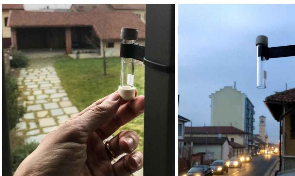
Figure 1. Passive sampler during installation (left) and operational (right) phases.
