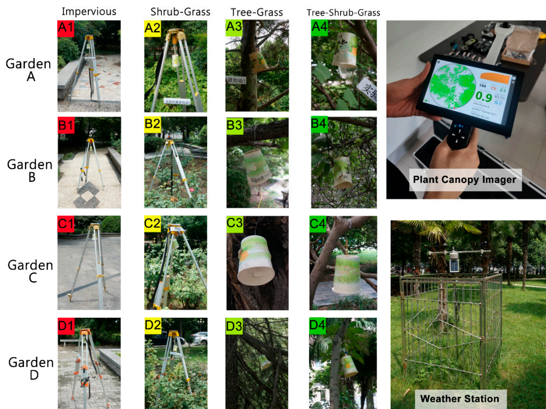
Figure 2. Sixteen measurement points in garden A, B, C, D; Plant canopy imager and weather station used in measurement.
