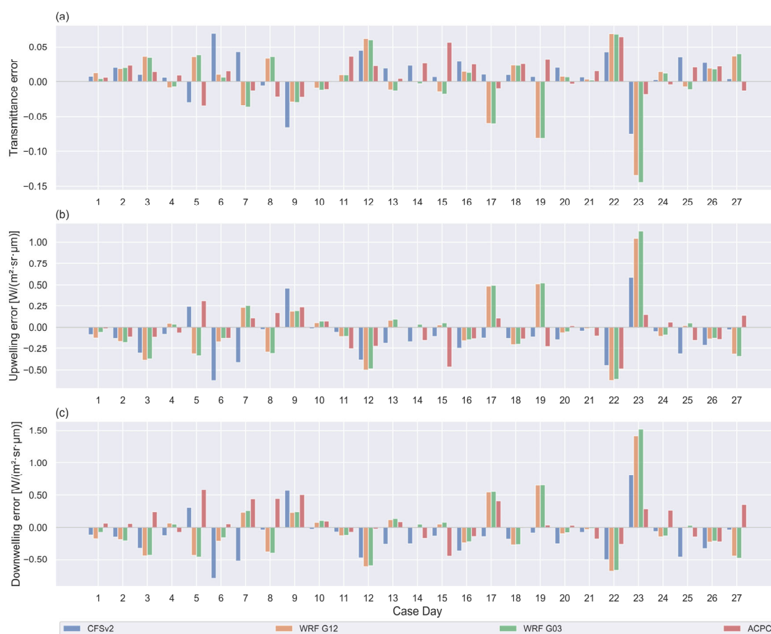
Figure 4. Errors in the estimation of (a) atmospheric transmittance, (b) upwelling radiance, and (c) downwelling radiance from the different profiles for each case day.
