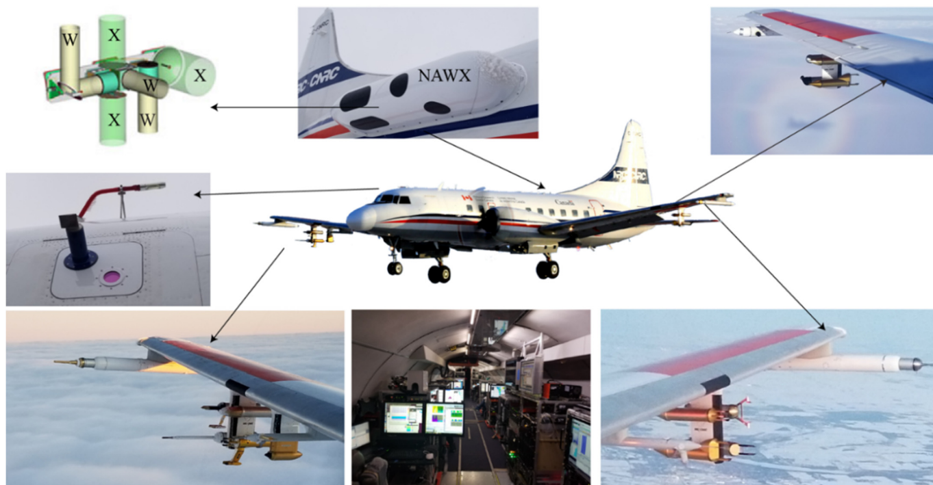
Figure 1. Illustration of the NRC Convair-580 aircraft instrumented for the ICICLE campaign in 2019, reproduced with permission from [24]. Top row: NRC's radar system (W- and X-band) and its axial pointing options and underwing cloud probes. Middle row: Aerosol isokinetic sampling inlet and bulk water detectors installed on the fuselage. Bottom row: Underwing cloud and atmospheric-state probes. Bottom middle: Cabin configuration with operator stations.
