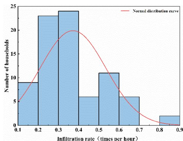
Figure 4. Distribution histogram of the infiltration rate.
