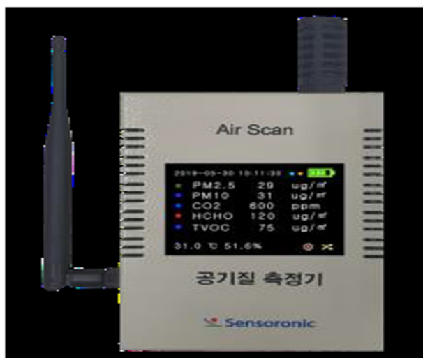
Figure 2. AirScan Device used for monitoring the Indoor Air Pollutant level.
