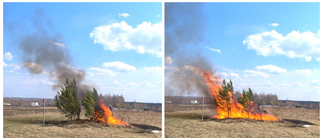
Figure 3. Image of the initial moment of a ground fire formation, and the transition of a ground fire to a crown fire.
