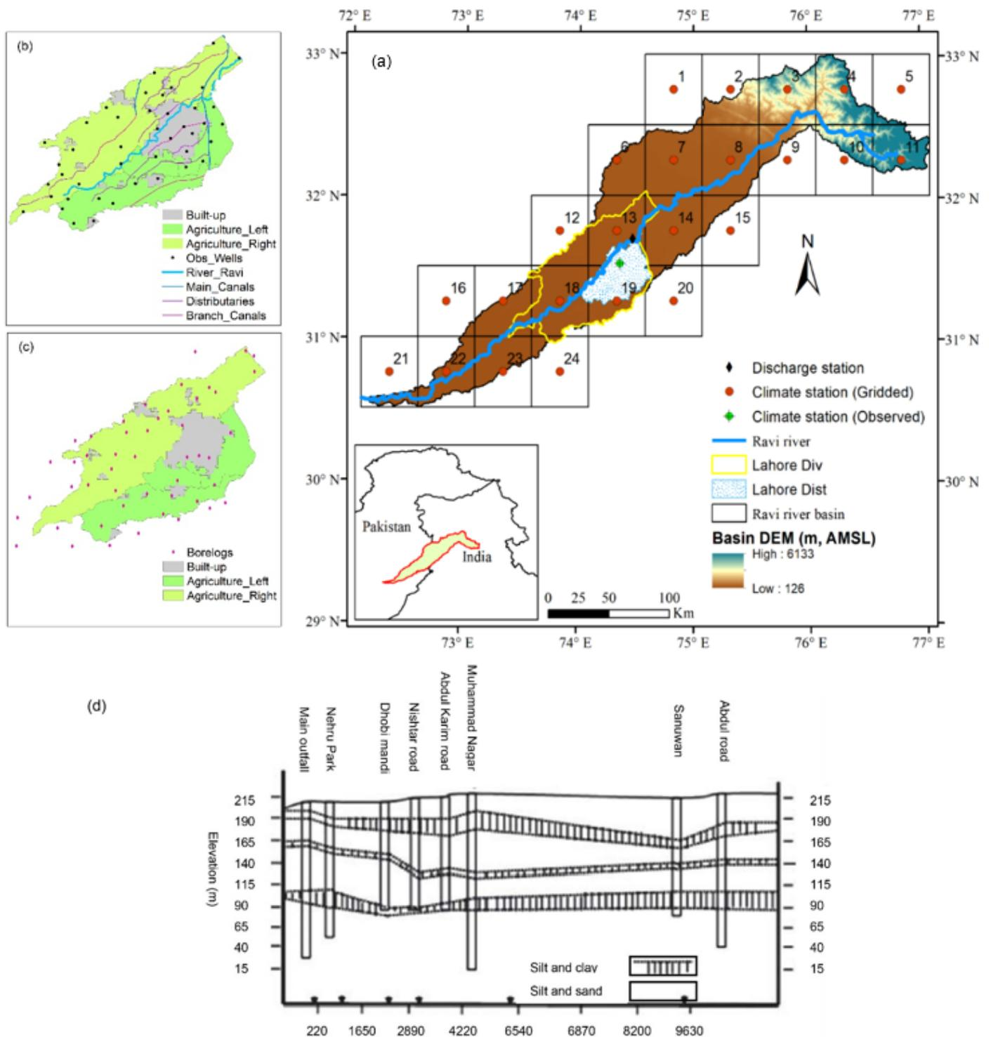
**Figure 1.** The geographic location of RRB. Topography is based on ASTER data. Climate stations (observed and virtual) are shown together with the  $0.5^\circ \times 0.5^\circ$  grid points (a). Three zones of Lahore division (Urban and Agriculture), river, canals, and observation wells are shown in (b). Bore-logs and their locations are shown in (c). Lithological classification of Lahore division aquifer in (d) [14].
