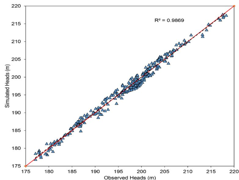
**Figure 7.** Scatter plot of the observed and simulated heads in Lahore.
