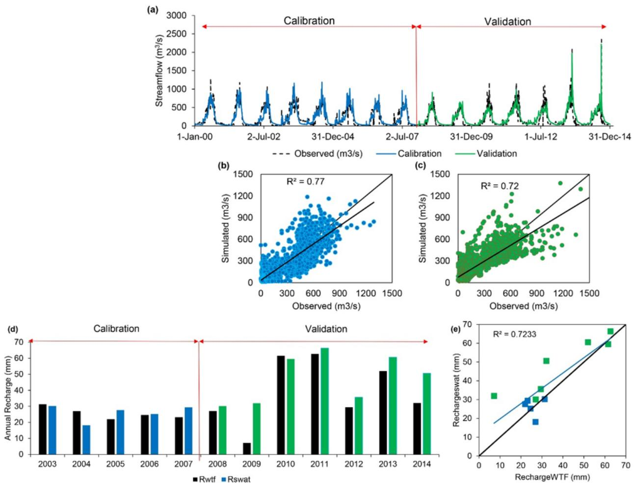
**Figure 4.** (a–c) Comparison between simulated and observed discharge for calibration and validation periods at Ravi siphon gauge based on daily time series and scatter plots; and (d,e) comparison between annual simulated and reference groundwater recharge for calibration and validation periods.
