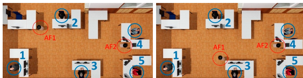
Figure 14. Geometry of baseline (left) and changed filter position (right). AF1: air filter 1, AF2: air filter 2. The numbering of the people locations in blue remain as previously.
