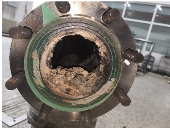
Figure 8. Precipitation and crystallization caused by urea injection in marine SCR system.
