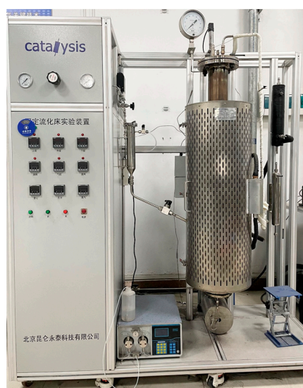
Figure S1. The fluidized bed reactor used in experiment
