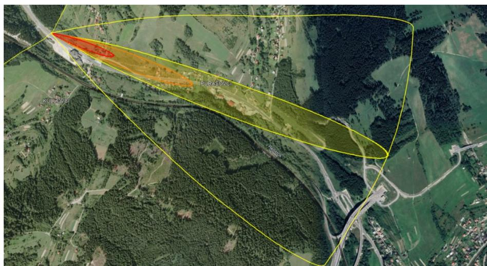
**Figure 6.** Graphical representation of the dispersion of a dangerous substance at the border crossing Svrčinovec-Mosty u Jablunkova [24,25].
