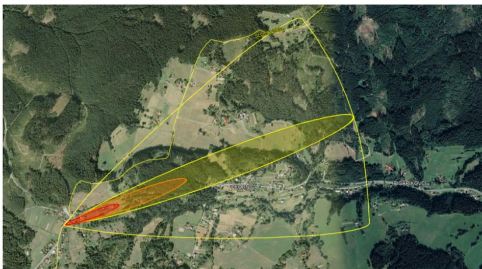
**Figure 4.** Graphical representation of the dispersion of a dangerous substance at the Klokočov-Bíla border crossing [24,25].
