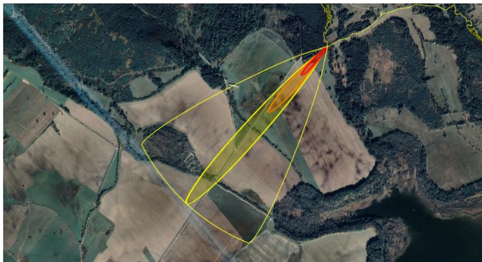
**Figure 11.** Graphical representation of the dispersion of a dangerous substance at the border crossing Bobrov-Wincerówka [24,25].
