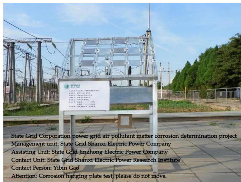
Figure 2. Diagram of hanging plate experimental device.
