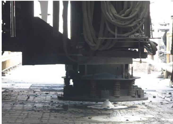
**Figure 6.** A charging telescope on the coal charging machine.
