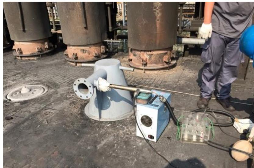
**Figure 5.** Self-designed closed sampling system for charge lid emissions.
