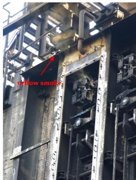
**Figure 3.** Yellow smoke containing VOCs was leaked out of the coke oven through its door gap.
