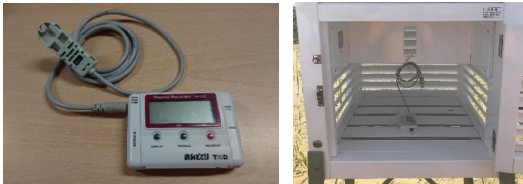
Figure 2. Installation status of the measuring equipment in the louver and temperature and humidity recorder, RH TR-72U.
