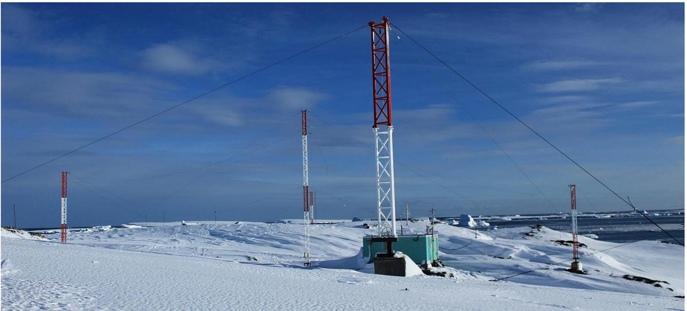
**Figure 4.** Antenna system of passive ionosonde at UAS.
