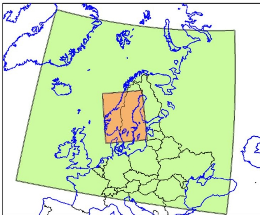
Figure 1. MATCH domains: in green covering part of Europe, with a 0.1^\circ \times 0.1^\circ grid cell size, and in orange the smaller domain at 4 \text{ km} \times 4 \text{ km} resolution covering Jämtland Härjedalen and surrounding areas.
