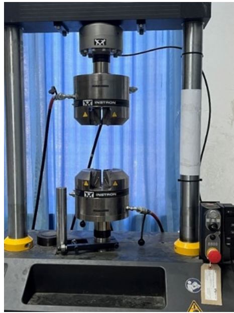
Figure 2. Instron 8801 electro-hydraulic servo fatigue testing machine.
