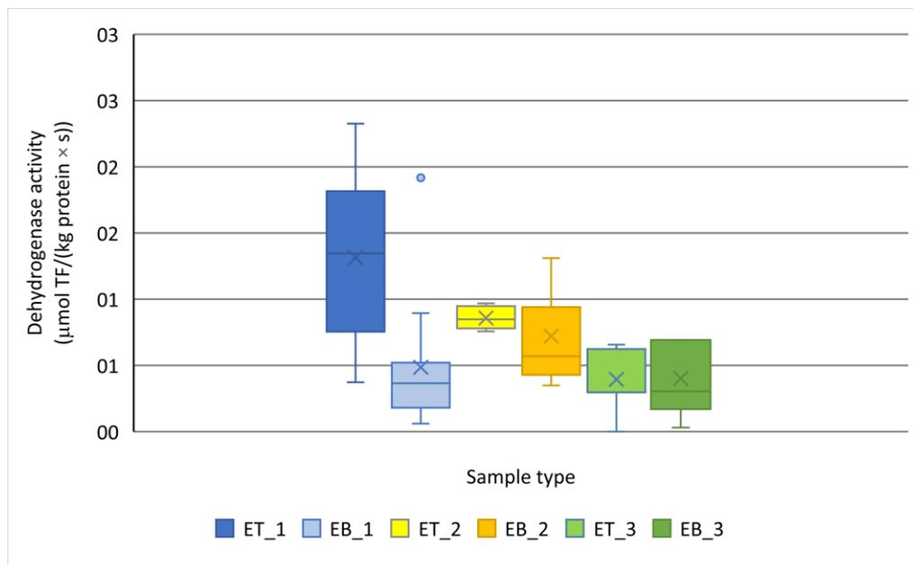
**Figure 4.** Dehydrogenase activity, endogenous samples. E—endogenous sample, T—top layer, B—bottom layer, 1—1st stage of experiment, 2—2nd stage of experiment, 3—3rd stage of experiment.
