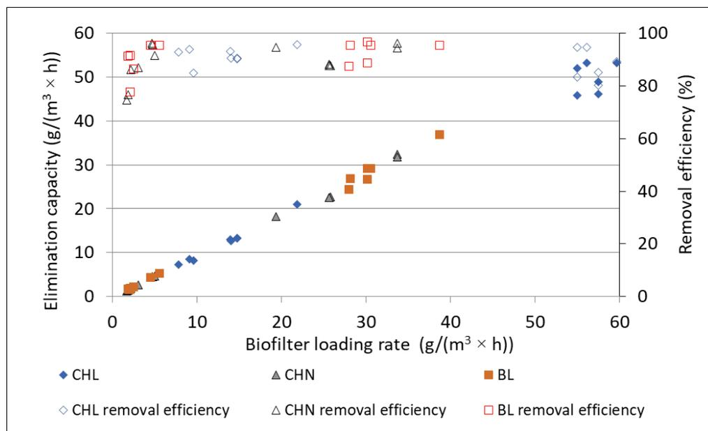
**Figure 2.** Elimination capacity vs. pollutant loading rate in the biofilter during the 1st, 2nd and 3rd stages of the experiment.
