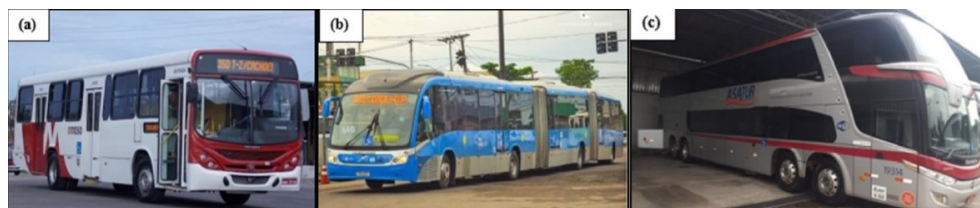
Figure 1. Illustrative images of the bus models used in this research. (a) Light Diesel Engine (LDV) for Urban Passenger Transport, (b) Heavy articulated bus (HDV) for urban passenger transport, (c) Heavy passenger intercity transport bus (HDV).
