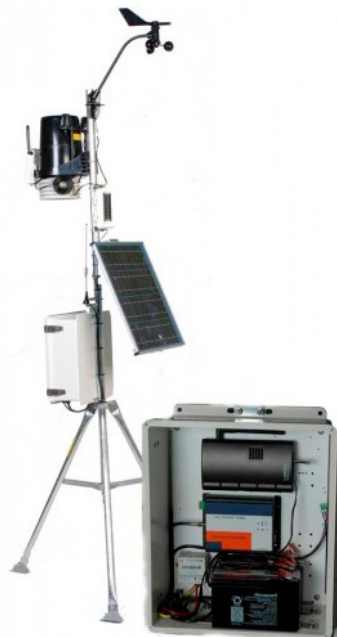
Figure 2. Automated weather station (AWS) for urban microclimate measurements.
