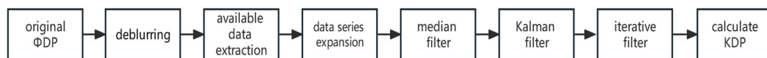
Figure 2. Flow chart for the quality control of the differential phase ( \Phi_{DP} ) and obtaining the specific differential phase ( K_{DP} ).
