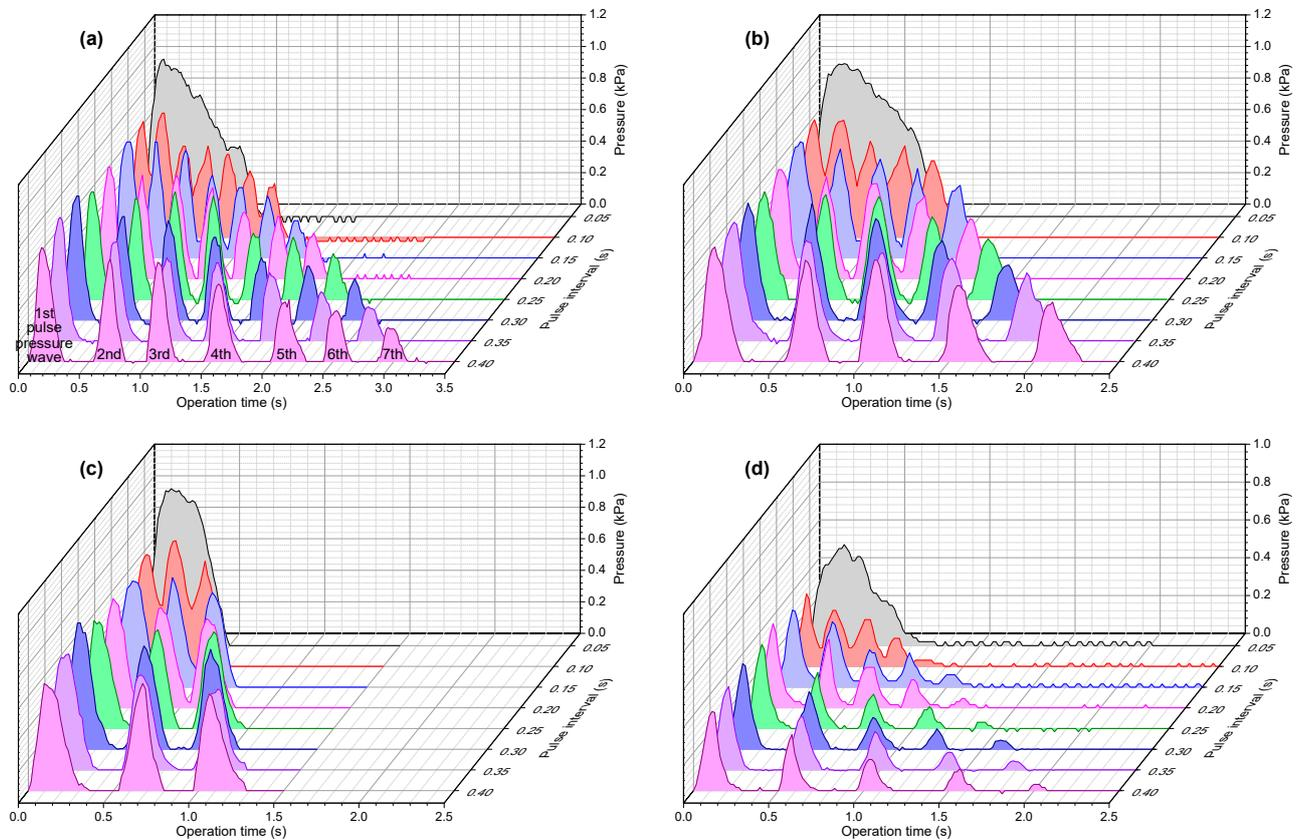
**Figure 5.** Pulse pressure on the inner surface of the filter during the (a) seven-pulsing, (b) five-pulsing, and (c) three-pulsing jet schemes in the offline cleaning modes, and (d) seven-pulsing jet scheme in the online cleaning mode with a pulse duration of 0.080 s and interval of 0.05–0.40 s.
