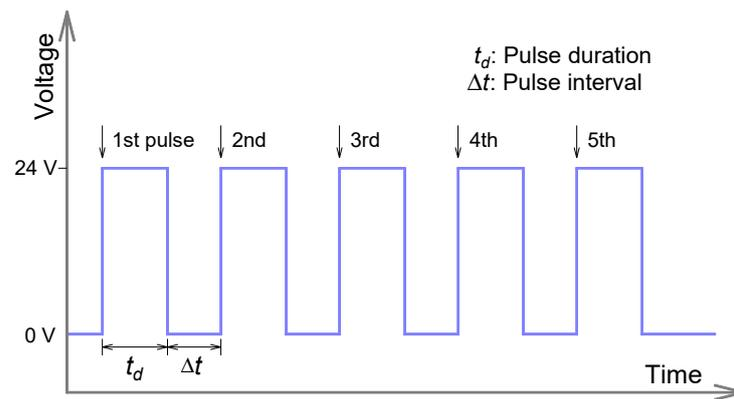
**Figure 2.** Diagram of the input signal for the magnetic valve in the multi-pulsing scheme.
