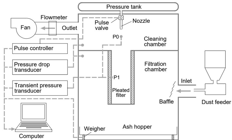
**Figure 1.** Schematic view of the test rig.
