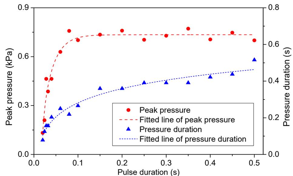
**Figure 4.** Peaks and durations of pulse pressures with varying pulse durations in the offline single-pulsing scheme.
