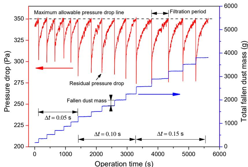
**Figure 6.** Evolutions of the filtration pressure drop and fallen dust mass under the five-pulsing jet scheme with a pulse duration  $t_d$  of 0.080 s and interval  $\Delta t$  of 0.05 to 0.15 s.
