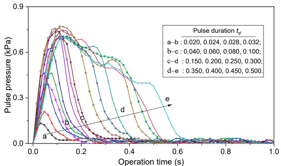
**Figure 3.** Evolution of the transient pulse pressure on the inner surface of the filter during a single-pulsing jet with pulse duration varying from 0.020 s to 0.500 s in offline cleaning mode.
