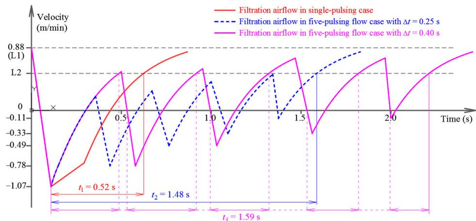
**Figure 8.** Comparison of the face velocities under the single- and multi-pulsing jet modes.
