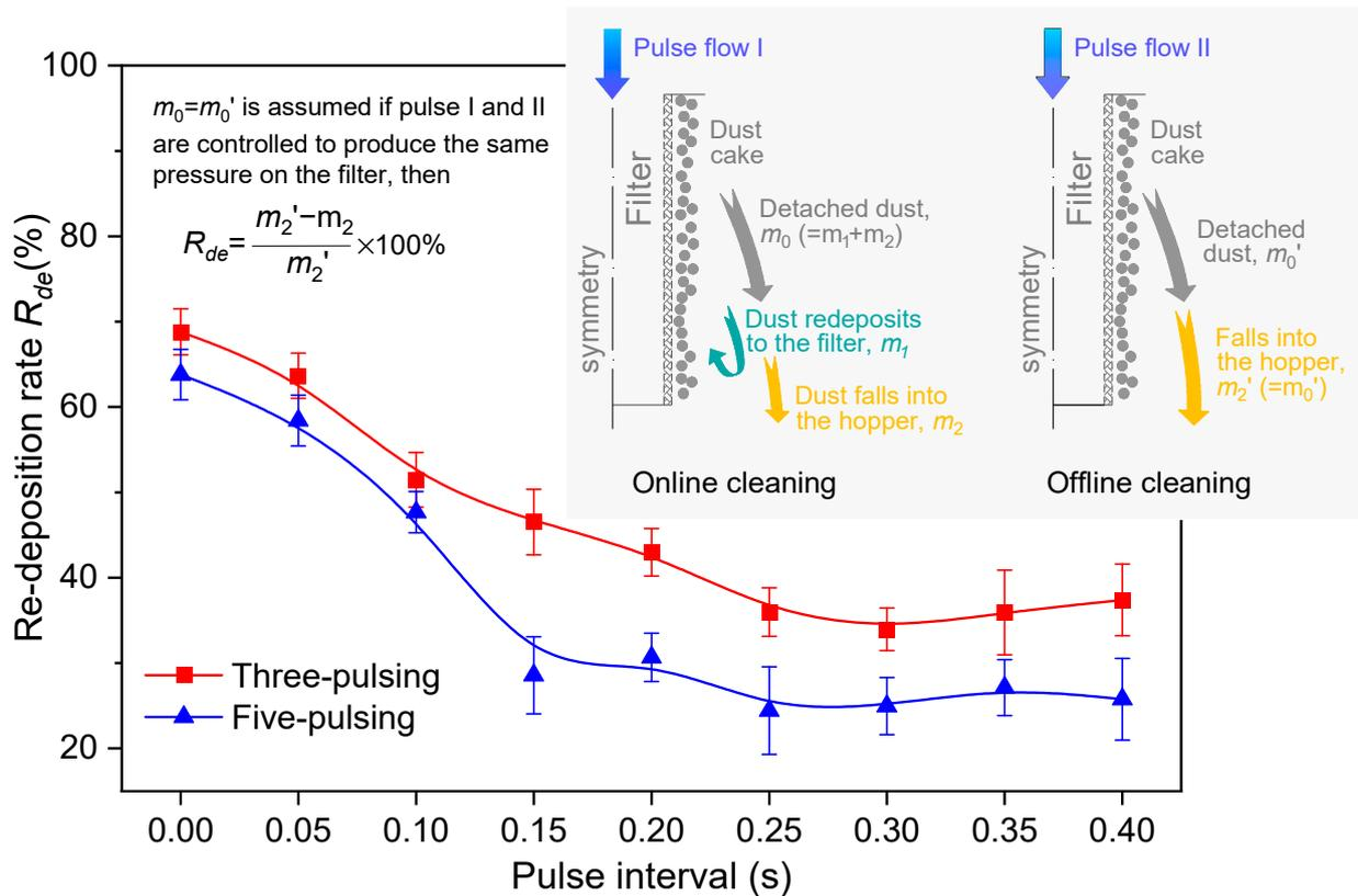
Figure 7. Re-deposition rate for three- and five-pulsing jet cleaning.
