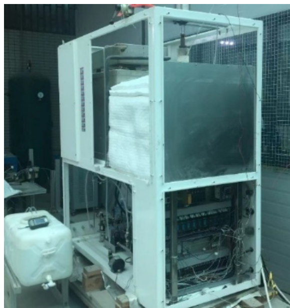
Figure 1. Physical diagram of the SOFC system.
