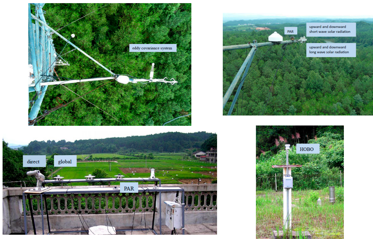
Figure 2. The eddy covariance (EC, up left ) and solar radiation measurement ( up right ) systems in Qianyanzhou subtropical coniferous forest operated by the Qianyanzhou experimental station. Another set of solar radiation (global radiation, direct radiation, and PAR) measurement systems ( bottom left ) located at a top of the building, and a HOBO weather station ( bottom right ) located at a meteorological observation station operated by Bai's group.
