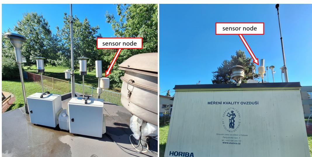
**Figure 1.** LCS sensor node placed on the roof of the reference air quality monitoring station of the health institute in Ostrava located in the Mariánské Hory district.
