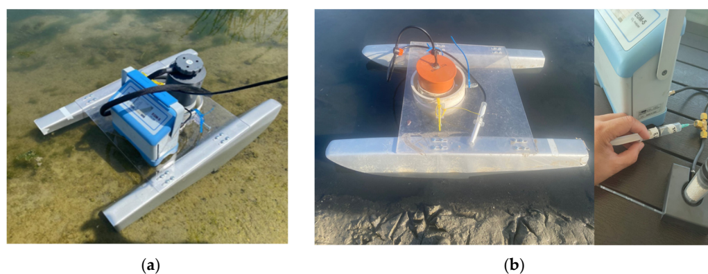
Figure 2. Field measurements with EGM-5 method on water (a) and the Injection Kit measurement method (b).
