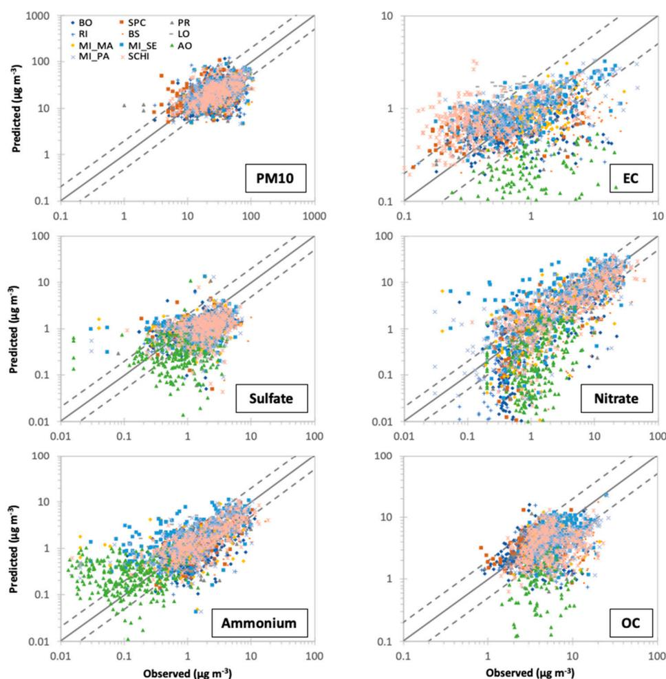
**Figure 6.** Comparison of predicted vs. observed PM<sub>10</sub> mass and PM<sub>10</sub>/PM<sub>2.5</sub> main chemical components concentrations ( $\mu\text{g m}^{-3}$ ) from 11 measurement stations in Northern Italy during 2019. Each point corresponds to a 1-day average value. Also shown are the 1:1, 2:1 and 1:2 lines. Observed data represent gravimetric and chemical measurements. Carried out by ARPAs on filter samples.
