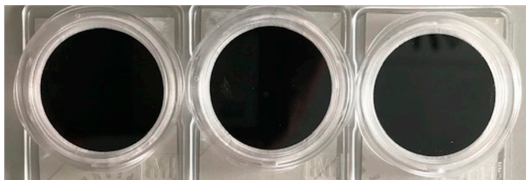
Figure 15. Image of three filters collected during PG42 brake emissions testing.
