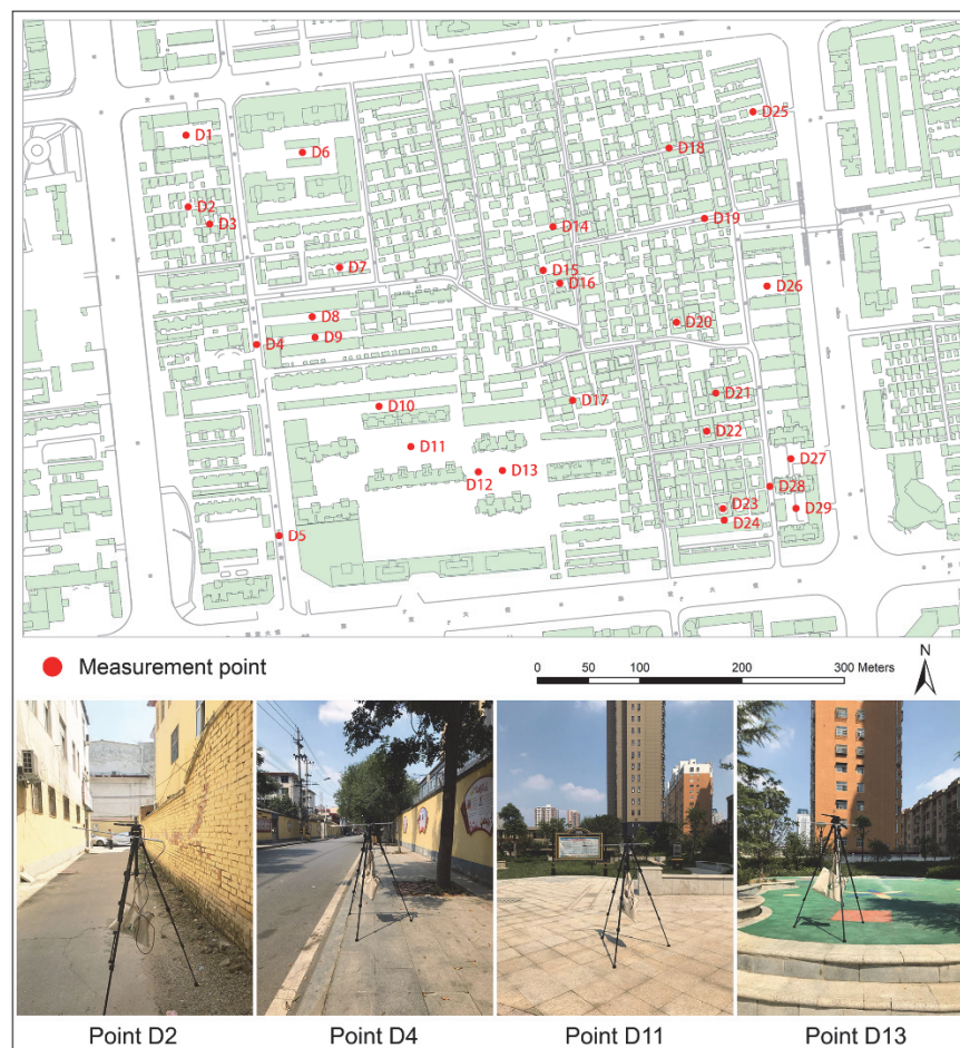
Figure 2. Spatial distribution of measurement points and instrument setup images in the demonstration blocks of the old district in Zhumadian City.
