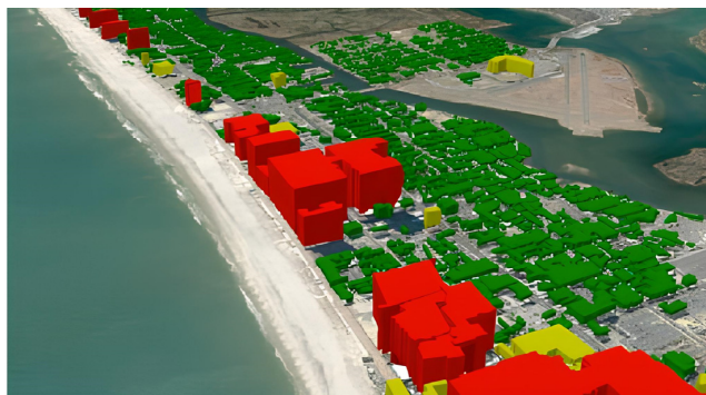
Figure 9. Three-dimensional depiction of the building structures derived from LiDAR data (Buildings are classified as high-rise (red—54.9 meters and above), mid-rise (yellow—54.9–29.3 meters), and low-rise (green—29.3 meters and below). (source: [60]).
