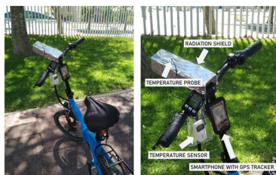
Figure 13. Equipment used for UHI study conducted by mobile measurement bicycle (source: [80]).
