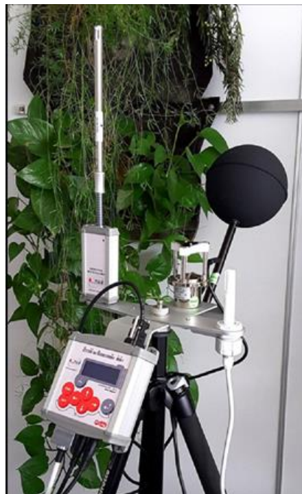
Figure S4. Microclimate control unit consists of M-Log, probes and supports
