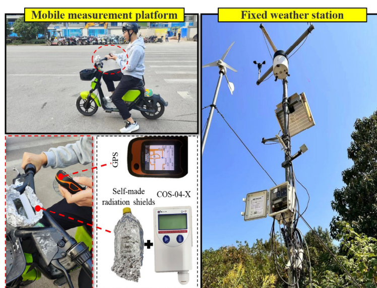
Figure 5. The setting of mobile measurements. The left half of the picture shows a mobile measuring platform; the right half of the picture shows a weather station.
