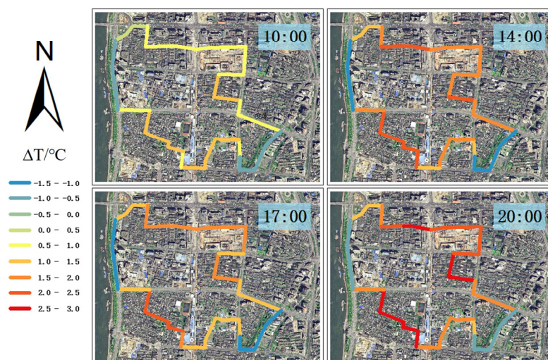
Figure 12. Distribution of temperature on mobile test routes. \Delta T denotes the temperature differences between the mobile route and the suburban area.
