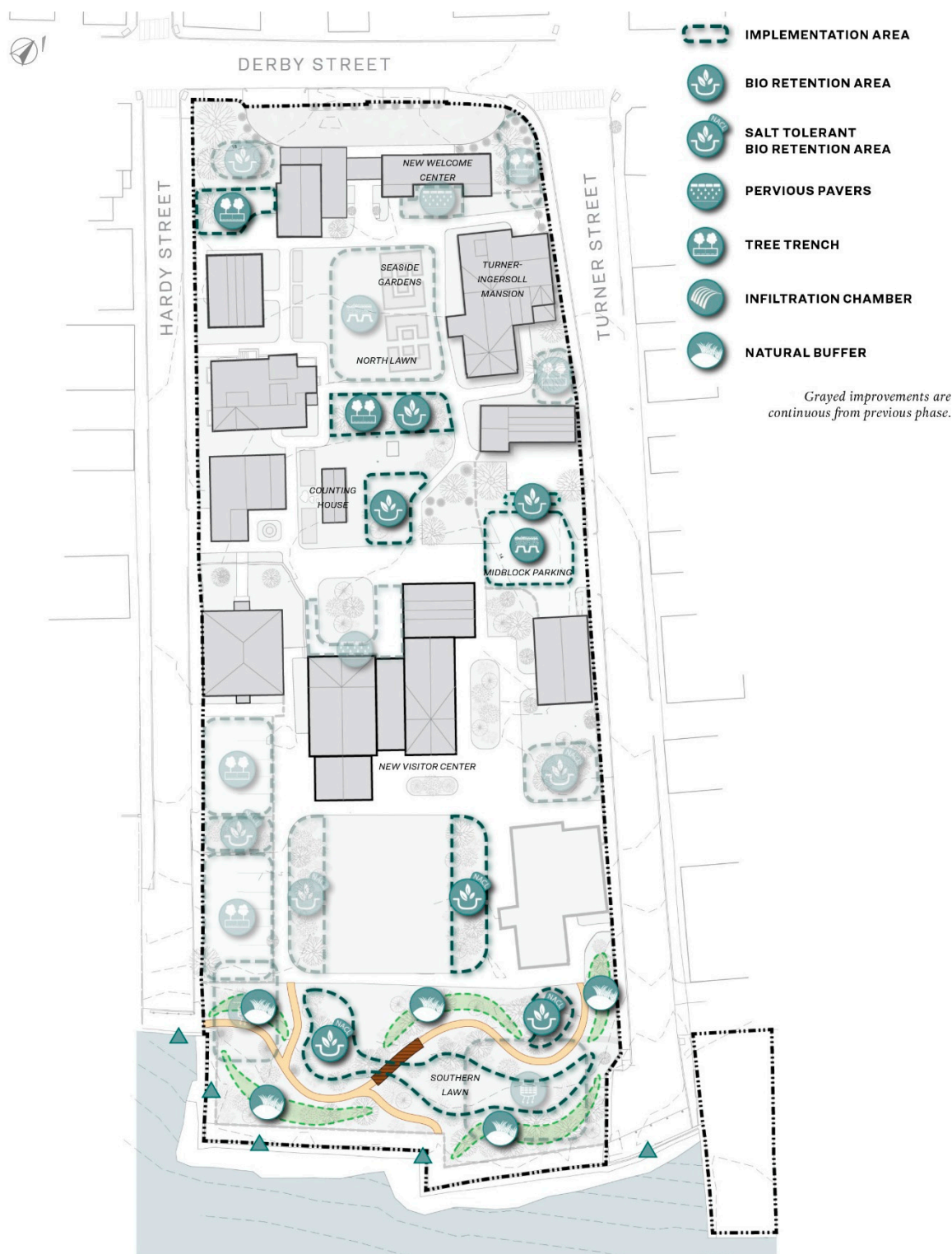
Figure 13. Proposed stormwater improvements in phase V [20]. Previous improvements from prior phases are shown grayed out but are still meant to be used. Drawing by the Horsley Witten Group.
