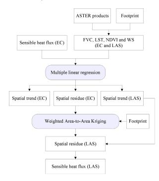
Figure 2. Process flowchart of WATA RK for sensible heat fluxes.
