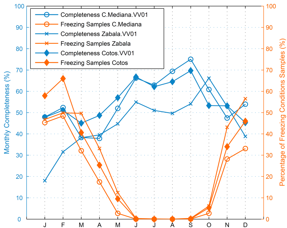
Figure 8. Data completeness (blue) for three sites and percentage of wind speed measurements taken under freezing conditions (orange).
