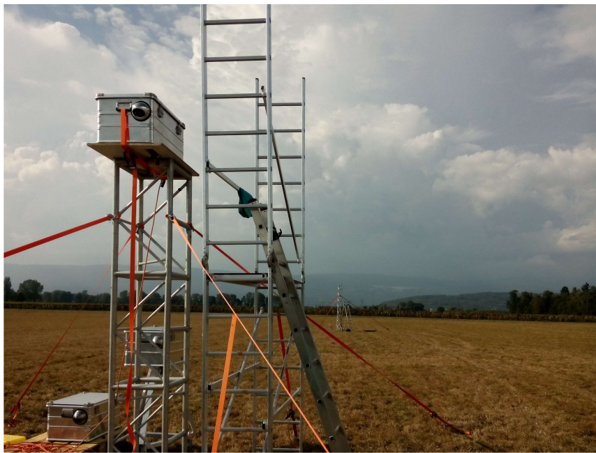
Figure 3. Three miniDOAS instruments located at the release site, 15 m downwind of the source center (position near ). The distances between the boxes containing the light source and the detector (picture foreground) and the reflectors (picture background) were approx. 35 m. The measurement heights were 0.5 m ( near / bottom ), 1.25 m ( near / middle ), and 3.0 m ( near / top ) above ground.
