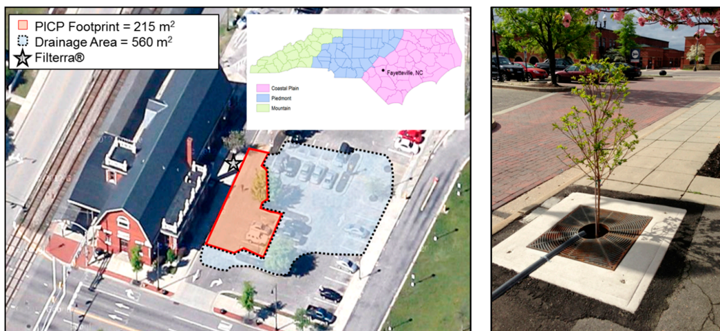
Figure 2. From left to right: Plan view of site with drainage areas and SCM locations, and PICP-FIL system. PICP (background) and Filterra ® (foreground).
