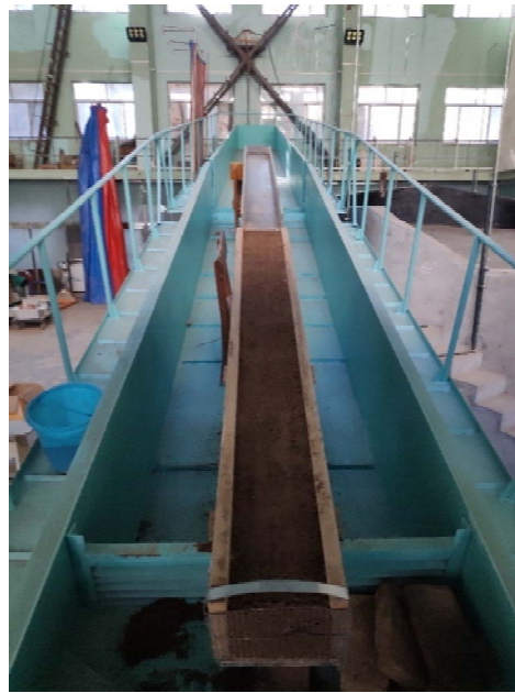
Figure 2. Photograph of the scouring experiment model.
