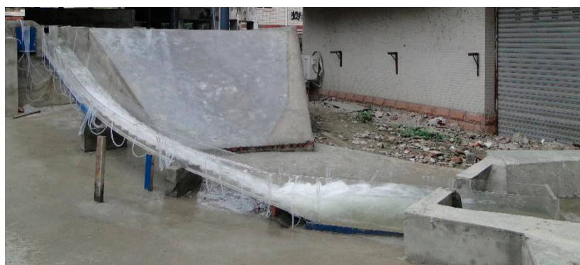
Figure 6. Flow pattern of the curved stepped spillway.
