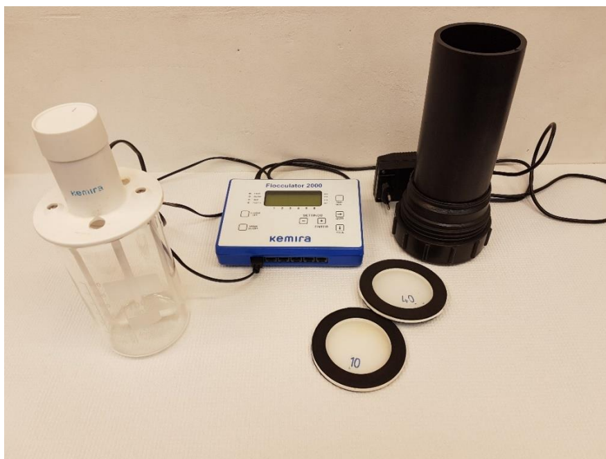
Figure 1. Photo of the Kemira Flocculator 2000 (Helsingborg, Sweden) and the laboratory-scale disc filters from Nordic Water.
