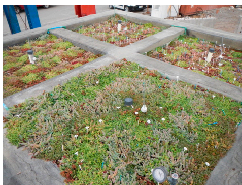
Figure 1. Photo of green roof specimens tested in the LIVE.
