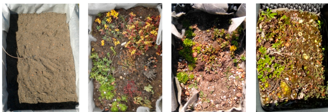
Figure 1. Long-term open air green roof experiment. Photos (from the left): first year (2013)—bare substrate; June 2015—model planted with Sedum plants; images from 2016 to 2017 (fifth year)—shows poor development of plant cover.
